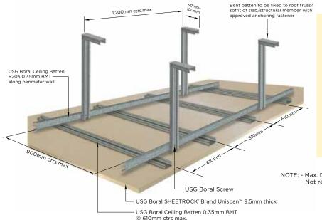
Metal Framing Members that Allows Maximum Spans When Used with USG Boral SHEETROCK® Brand Unispan<sup>™</sup> 9.5mm Plasterboard
