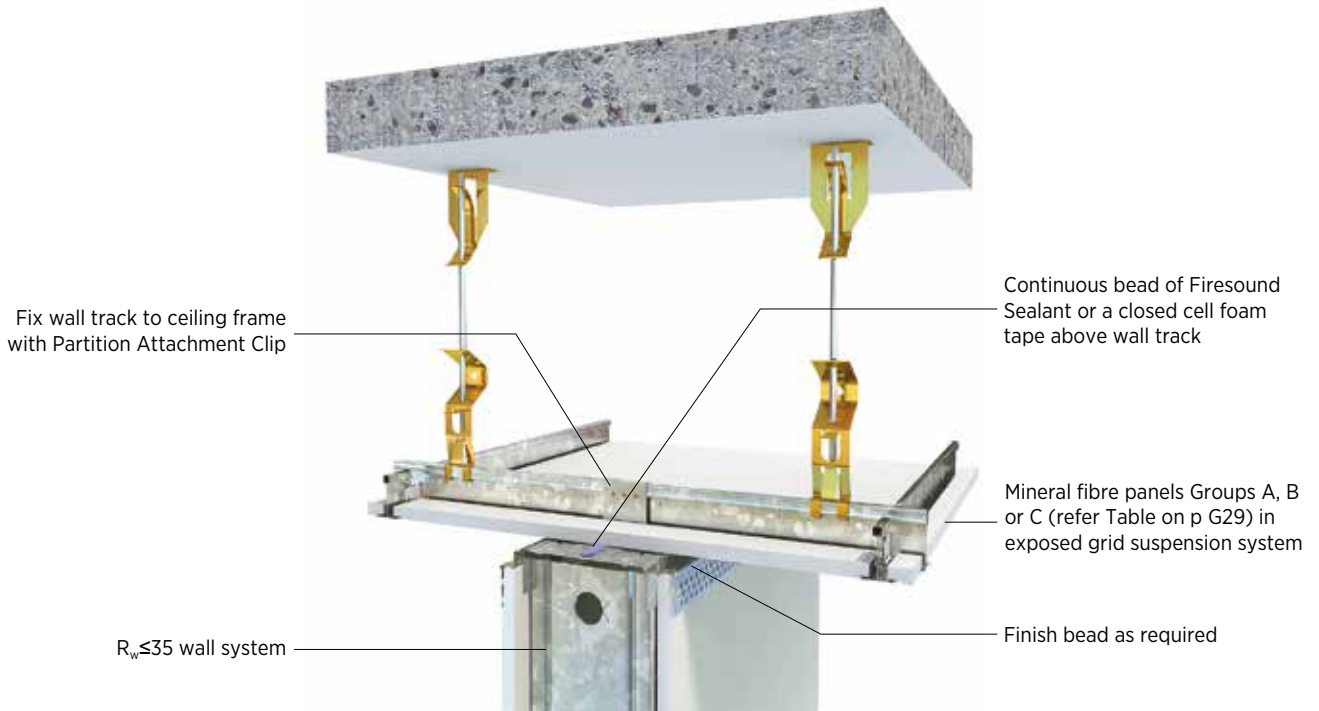
Figure G12: Ceiling configuration to maintain an R_w \leq 35 wall acoustic rating (System OP.1 shown)
